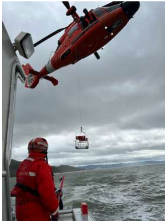
Alex Bennett, FI 14, grasps the grounding rod to dissipate the residual electrical charge from the hoist basket of the ASSF M-65 helicopter.
