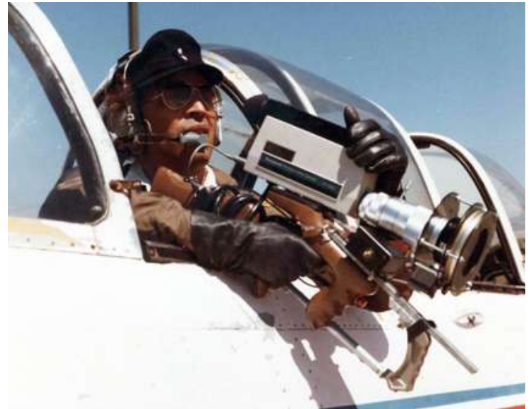
Bill Burns holding a Light Airborne Oil Surveillance System test unit. Photo by Bill Burns.
