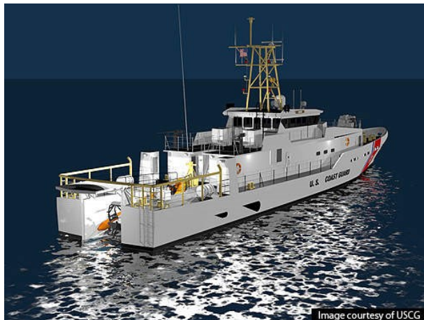
Left Photo: FRC Sentinel Class stern launch capability Right Photo: Underway with 28 knot capabilities - Photos USCG and Bollinger Shipyards
