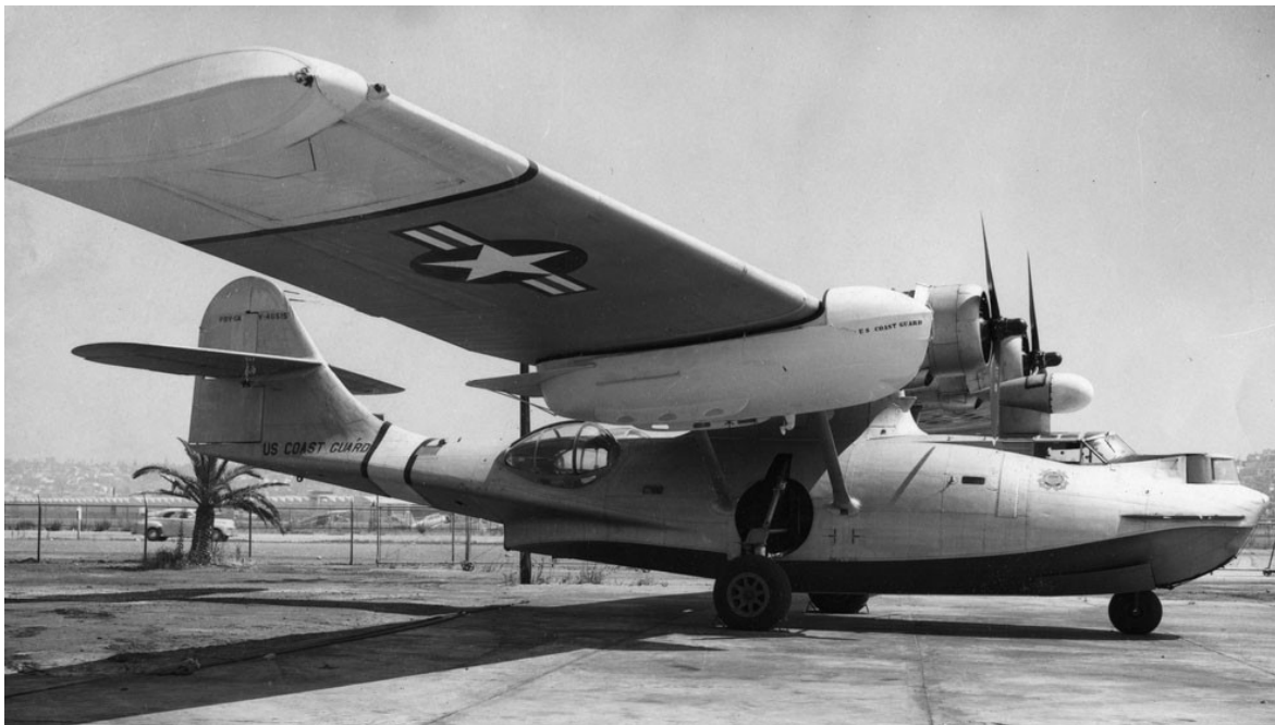
USCG PBY-5A on the ramp with airborne droppable life boat attached - Photo: USCG
