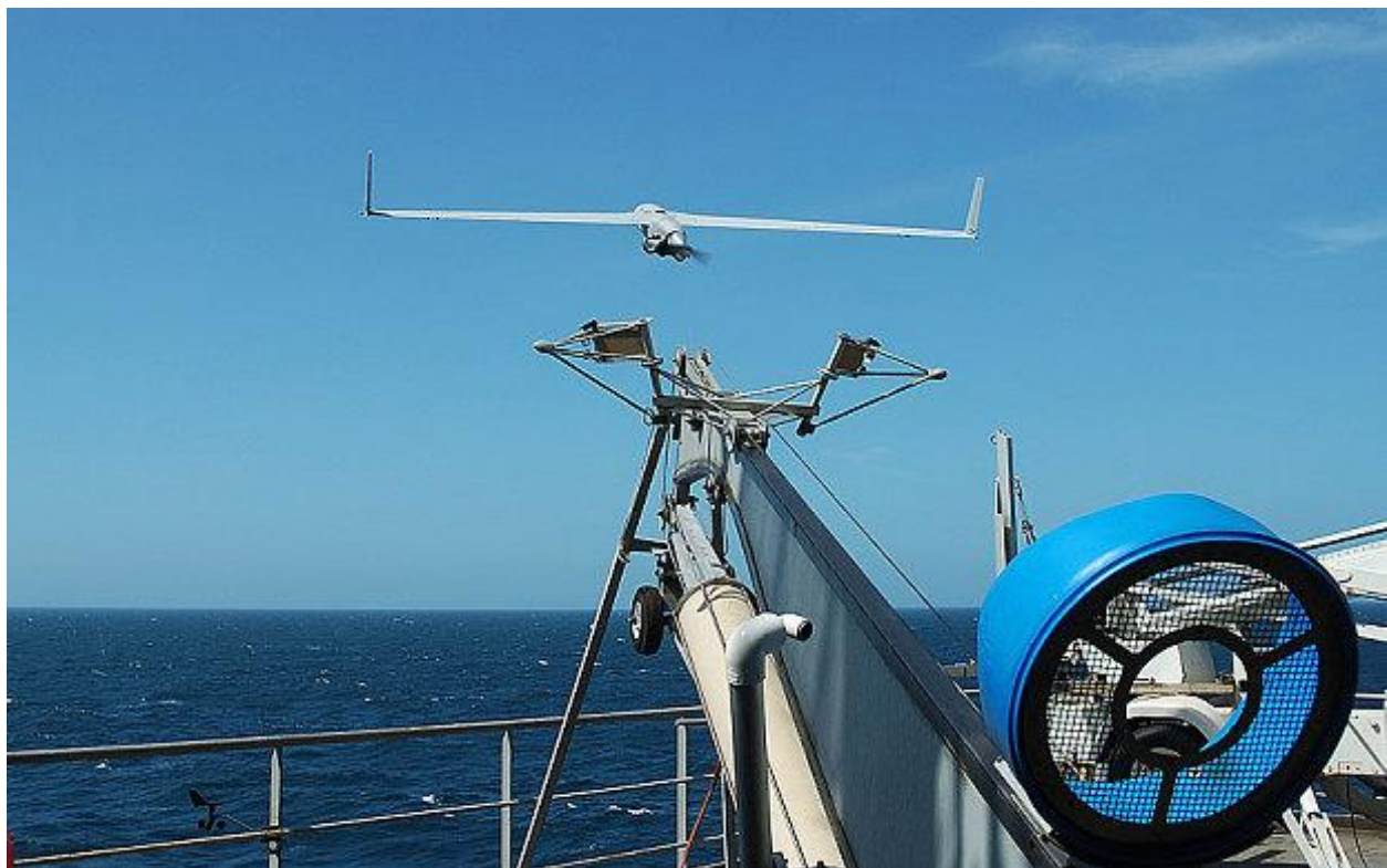
ScanEagle Launched for Flight is fitted with a pusher engine and a two-blade propeller – Photos: Insitu, Inc.
