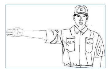
Move vehicle in direction indicated using flashlight in low visibility situations. Signal indicates trailer or vehicle end needs to move left or right not that driver is to turn vehicle's wheels.
